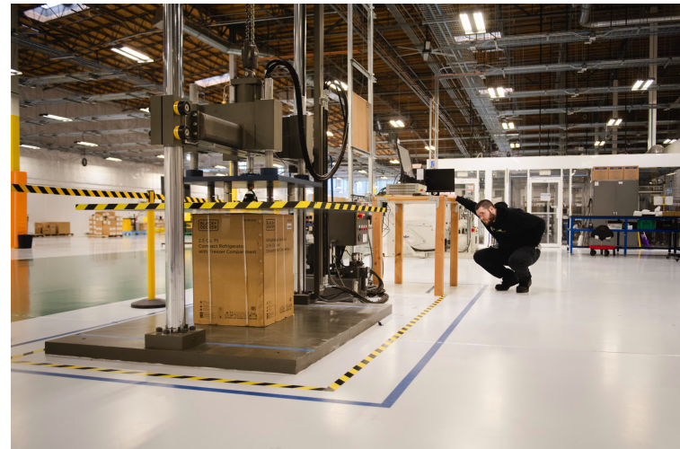
At its testing facility in Sumner, Wash., Amazon tests if packages can survive delivery unscathed. This Compression Tester simulates stacking in vertical compression, explained Rett Bruce, a senior lab technician. PHOTO: KHOLOOD EID FOR THE WALL STREET JOURNAL
